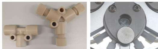
Figure 10. Types of mixers including T-piece and arrowhead mixers, in addition to a CSTR stages with cross stirrer (left to right). 95
